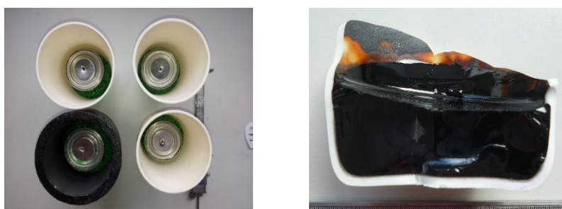
Fig1: (Left) Laboratory scale PCM mock up drums, with addition of 1.04 wt% CeO 2 , as a Pu surrogate. (Center) Addition of glass forming frit at a 1:1wt% ratio with waste simulants. Thermal treatment 1560°C Melting temperature for 4 hours. (Right) example of vitrified waste product, masonry in this case.
