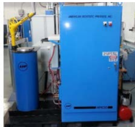
The University of Sheffield's research scale hot isostatic pressing facility.
