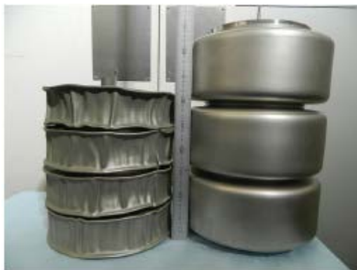
An example of the volume reduction achievable by hot isostatic pressing.
